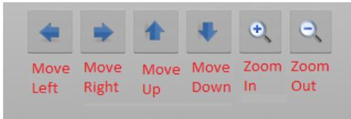
If camera PTZ is enabled in VMS Server, then PTZ buttons are displayed in as shown. User can press the button to pan / tilt/ zoom the camera.
